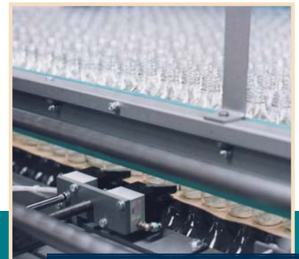
Friction plates plus tier sheet grippers stabilize the secondary layer during sweep off.
