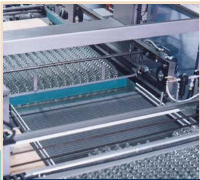
Elimination of "sweep off gap" keeps bottles stable from pallet to discharge.
