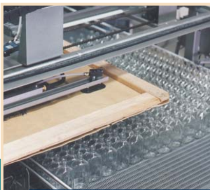
Picture frame and slipsheet removal and stacking are automatic.
