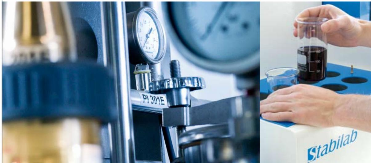
**C**enodia uses the same technology for both tartrate stabilization and acidification, namely electrodialysis. This has already been tried and tested in many other fields such as green chemistry and the sugar and dairy industries. However, Cenodia is currently the only company in the world to apply this technology successfully to wine production.
